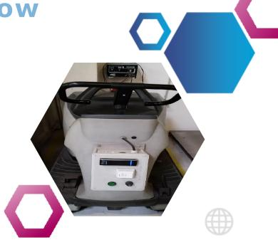
a security software from Elo. This software solution is comprehensive to the extent that allows the managers to access data of those who used the equipment and when they did so. So whenever an employee uses a forklift or other equipment, a registration and date when the device was used is recorded.
